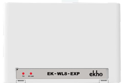
Any combination of Ekho wireless devices can be connected to the Expander Module\*. The Expander Module transmits the intelligent device information from the field devices to the Loop Translator Module using a highly stable bi-directional radio communication protocol. The system parameters are programmed into the Expander Module via the Translator Module.
