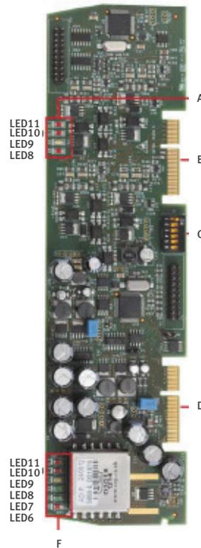
The card also monitors loop device status and provides status to the LCD Main Processor Board. It holds all device configurations and operates in a standalone manner where catastrophic failures occur.
