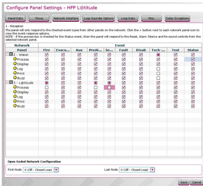
Flexible network configuration options using simple to follow PC configuration programme.
