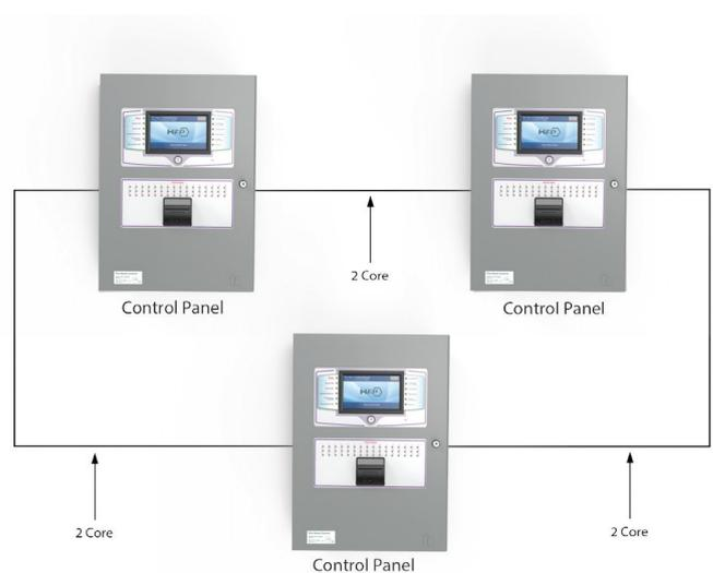
Two core loop wiring ensures network integrity by providing full isolation of faulty wiring segments.
